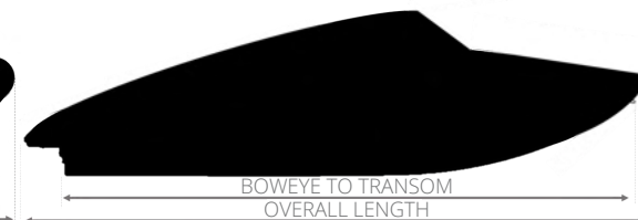
MOTORBOAT TRAILER MEASUREMENTS
